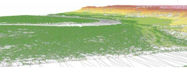
LandScape provides an advanced and efficient portal into the world of 3-dimensional LiDAR points. It edits large terrain point clouds such as LiDAR and offers tools for viewing stereo imagery, classifying and modifying 3D points (point clouds), and generating new data based on points. LandScape's tools can be configured by the user to enhance understanding of the data view.
