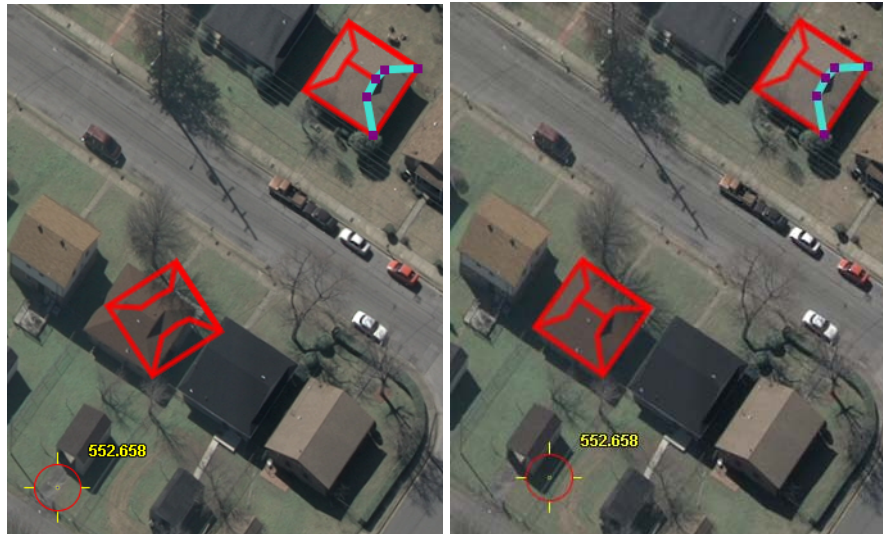
CRSELECTION shows some of the selected elements as transients during placement; all the selected elements are copied when the final angle is selected.
