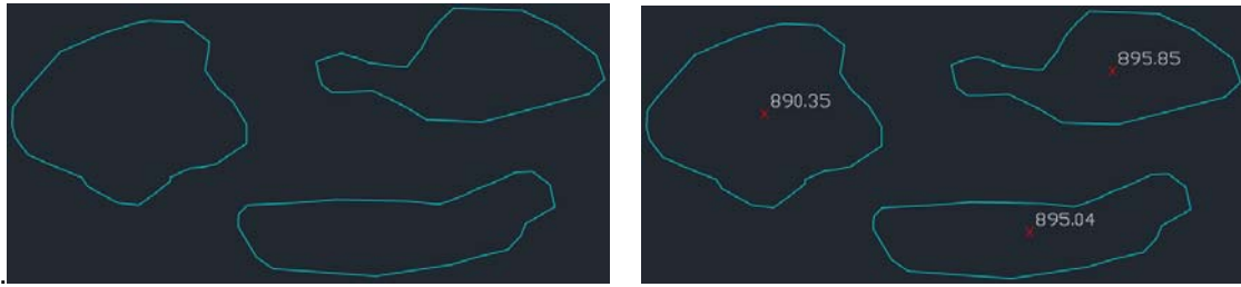
Before and after “Add Z Text or Block” adds blocks and elevation labels to closed polylines
