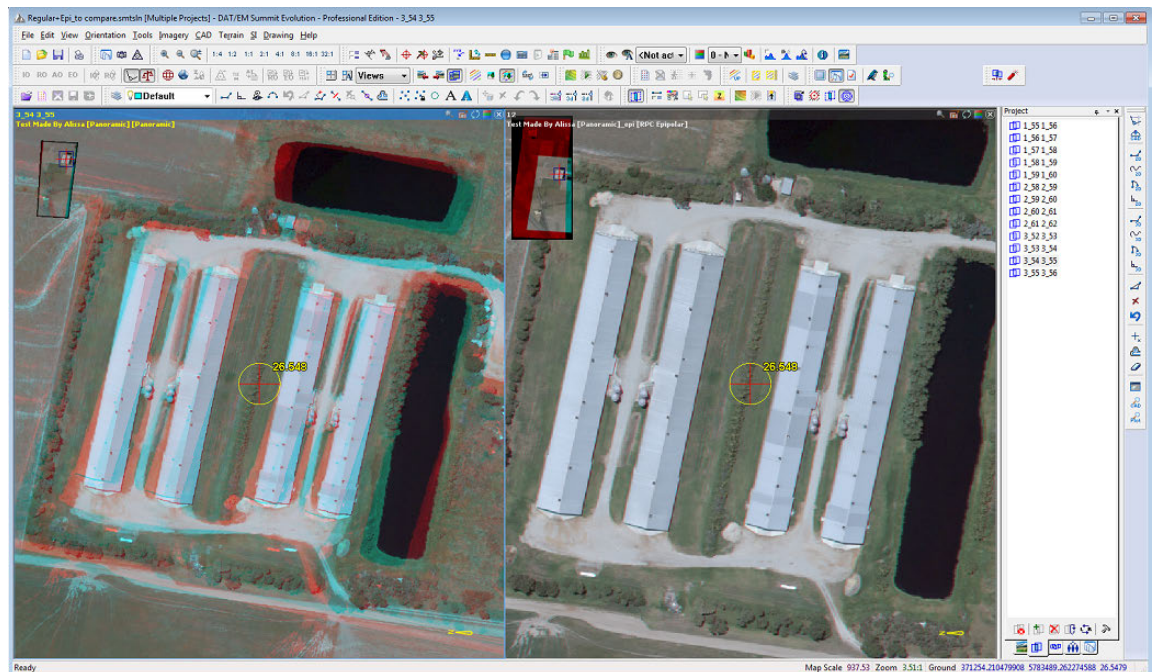
A3 Quasi-Panoramic "odd model" before epipolarization (left) and after (right) shown in a Summit Solution .smtsIn file with two open viewports
